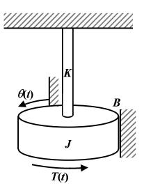
When T(t) is applied, friction and the spring will resist any motion so that, according to Newton's Second Law of Motion,
