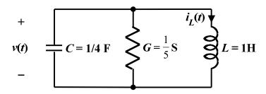
As shown by equation (1.7), this parallel RLC circuit can be described by the equation
