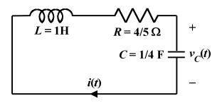
As shown by equation (1.16), this series RLC circuit can be described by the equation
