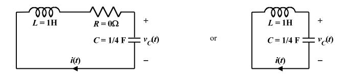
As shown by equation (1.16), this series RLC circuit can be described by the equation
