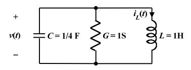
As shown by equation (1.7), this parallel circuit can be described by the equation
