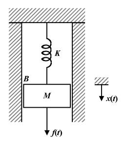
When f(t) is applied, friction and the spring will resist any motion so that, according to Newton's Second Law of Motion,
