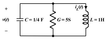
As shown by equation (1.7), this parallel RLC circuit can be described by the equation
